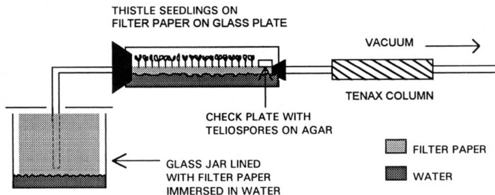
**Figure 1.** Diagram of apparatus for collecting volatiles from germinating thistle seeds.
